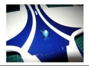
Glue the upper vertical fuselage halve onto the horizontal fuselage. Make sure it is perpendicular to the horizontal fuselage.
