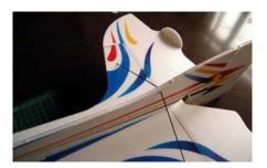
Mount the horns, landing gear, and pushrods. (Attention: scissor a jag on the horns and servo arms, glue with 502 bond where the horns and the pushrod join. The length of pushrods is subject to the actual assembly.)
